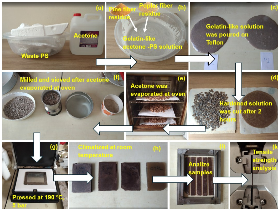
Fig. 1. Sample preparation process, waste PS and acetone solvent (a); PS in a gel-like state (b); gel-like blend (c); at room temperature (d); evaporation at oven (e); granulated and sieved samples (f); hot press (g); samples after pressing (h); analysis samples (i), TS analysis (k)
