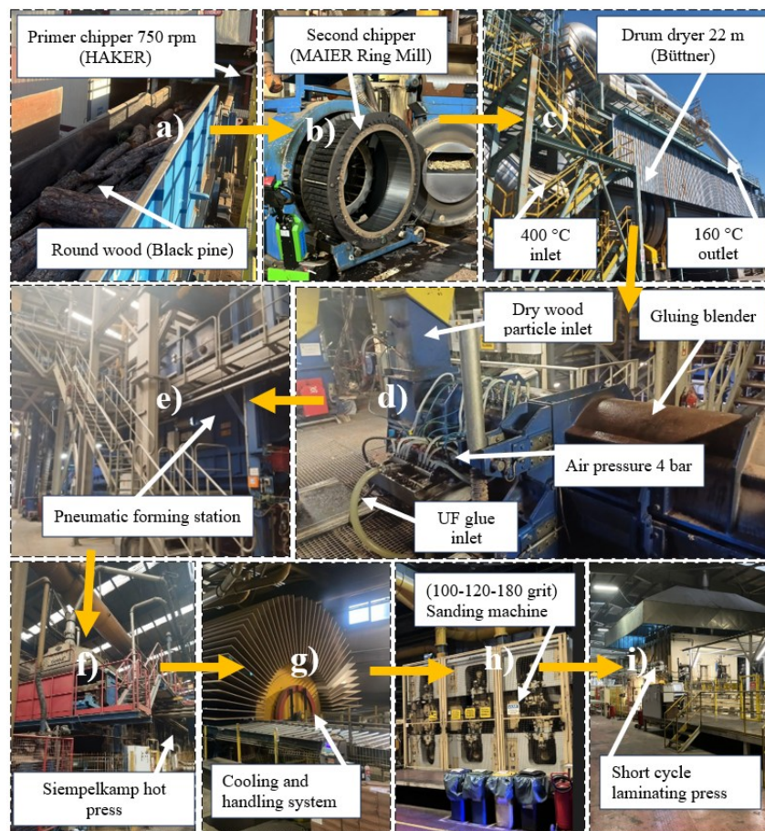
Fig. 1. Samples prepared at a real manufacturing line in Bolu province/Turkey; a) primer chipper, b) second chipper, c) drying, d) gluing, e) forming, f) pressing, g) climatizing, h) sanding, and i) laminating station.
