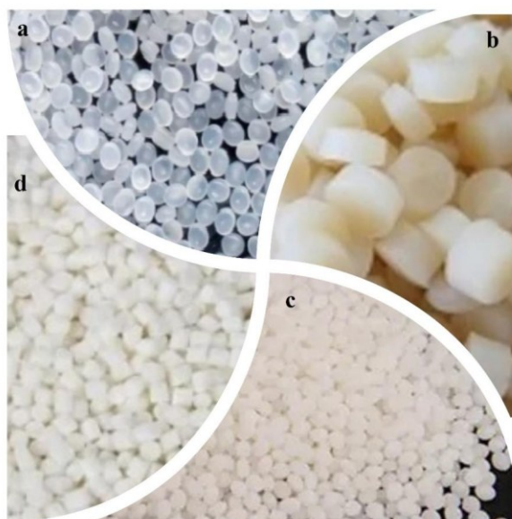
Fig. 2. Types of bio polymer pellets: (a) PLA, (b) PHA, (c) Starch, and (d) PCL
