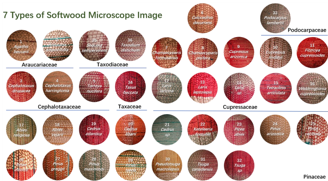
Fig. 1. The transverse section of 36 softwood species
