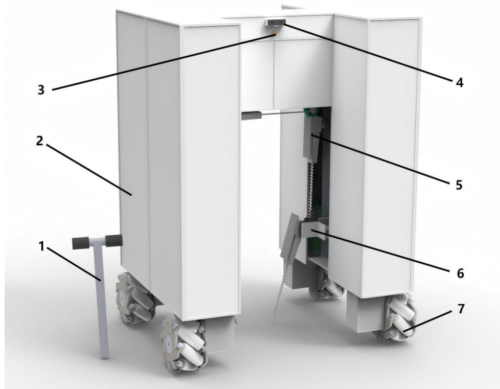
Fig. 1. 3D model of holly pruning machine with adaptive tool adjustment: (1) hand lever; (2) frame; (3) spraying mechanism; (4) vision mechanism; (5) pruning mechanism; (6) tool adaptive adjustment mechanism; (7) walking mechanism
