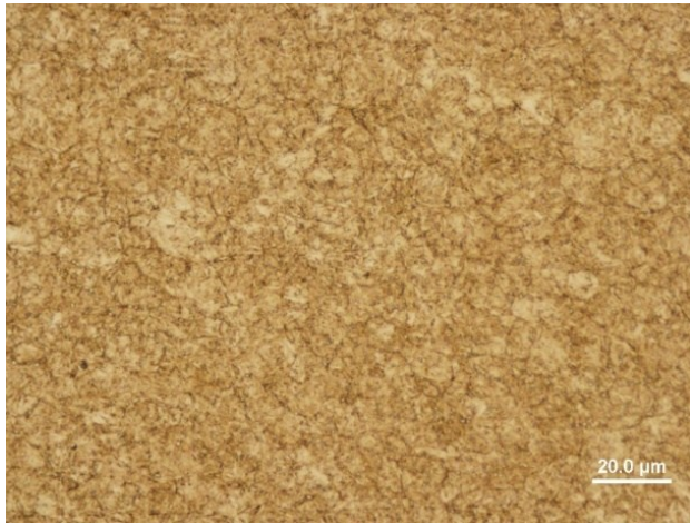
Fig. 2. Microstructure of X48CrMoV8-1-1 tool steel in “Condition 1”, i.e. , hardened and tempered material state without chemical-thermal surface treatment
