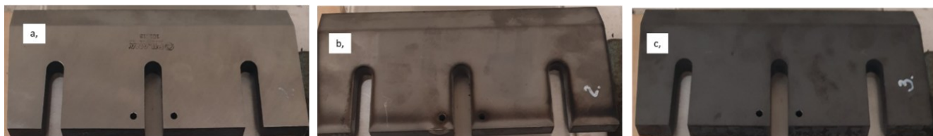
Fig. 1. Experimental chipping knives: knife in “Condition 1” - unmodified (a), knife in “Condition 2” - plasma nitrided (b), knife in “Condition 3” – PVD-coated with CROSAL ® Plus (c)
