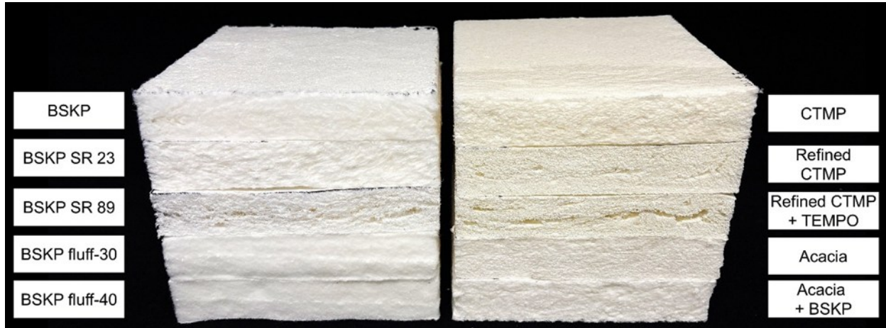
Fig. 7. Cross-sections of various samples. Those containing BSKP fluff were prepared by air-laying, while all the others were foam-formed. There are five samples in each stack. The target shape of the samples was a rectangular prism.
