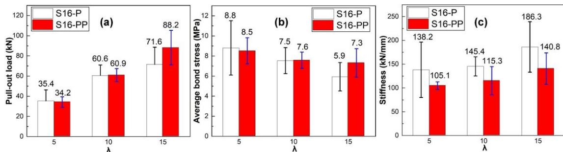
**Fig. 7.** Connection behavior of specimens with different rod-to-grain angle: (a) pull-out load; (b) average bond stress; and (c) stiffness.
