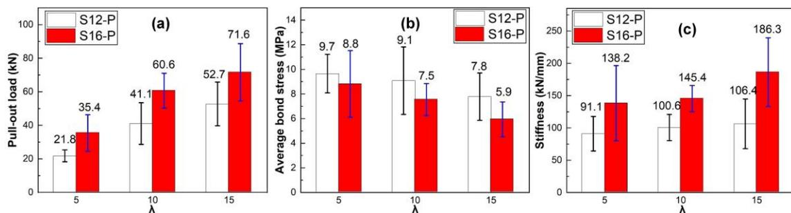
**Fig. 8.** Connection behavior of specimens with different rod diameter: (a) Pull-out load; (b) Average bond stress; and (c) Stiffness.
