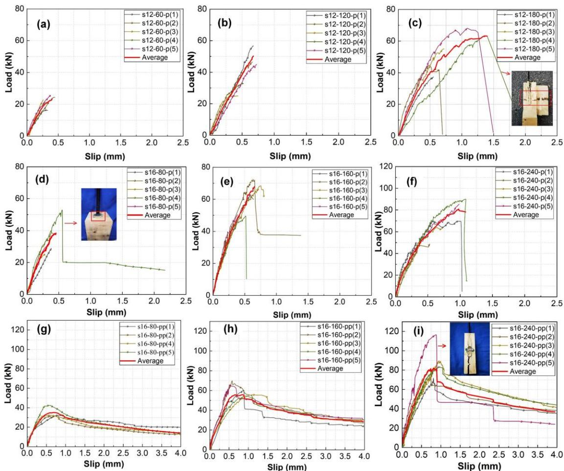
**Fig. 5.** Load-slip curves: (a) S12-60-P; (b) S12-120-P; (c) S12-180-P; (d) S16-80-P; (e) S16-160-P; (f) S16-240-P; (g) S16-80-PP; (h) S16-160-PP; and (i) S16-240-PP
