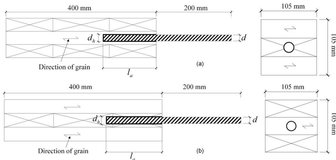
**Fig. 2.** Schematic diagram of specimen: (a) Parallel to the grain; and (b) perpendicular to the grain.
