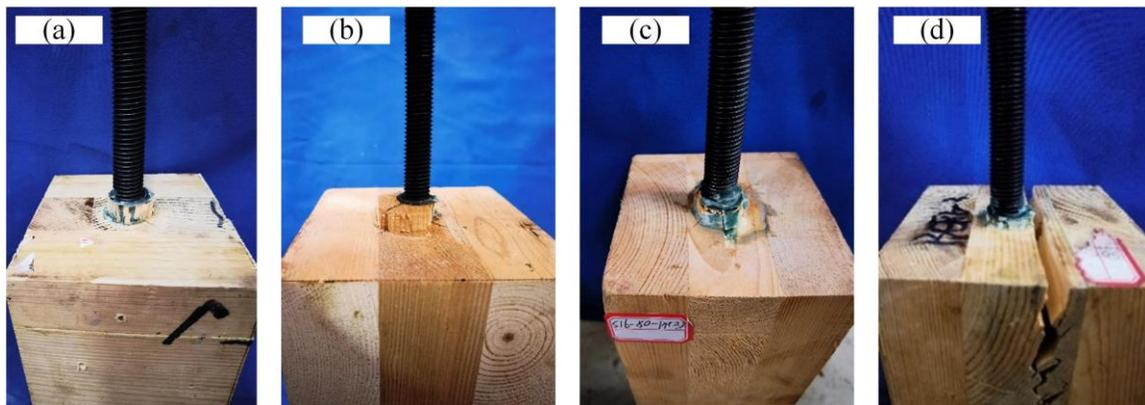
**Fig. 4.** Typical failure modes of specimens: (a) Timber-adhesive interface shear failure; (b) plug pull-out failure of timber; (c) mixed failure combining shear failure of adhesive layer and timber shear failure; and (d) splitting failure of the cross layer in CLT
