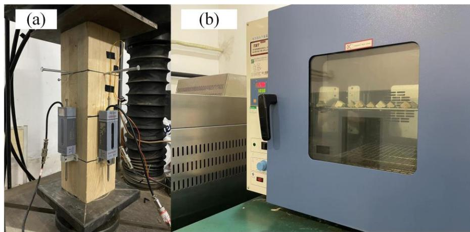
Fig. 1. Test diagram of CLT specimen: (a) compression test; and (b) Moisture content test
