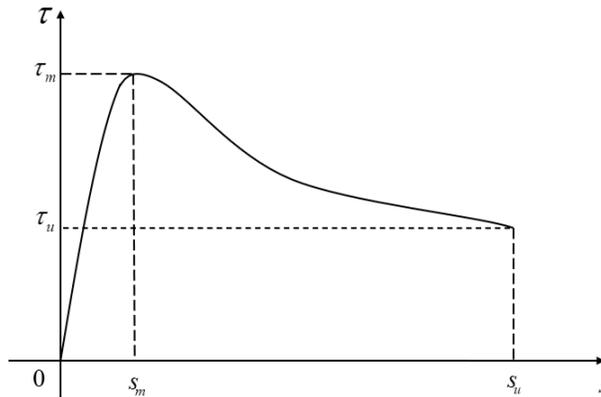
**Fig. 9.** Partially modified BPE model by Ling *et al.* (2014)
