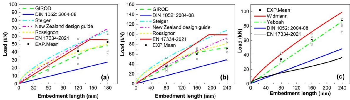
**Fig. 11.** Comparison between experimental results and the theoretical predictions: (a) S12-P series; (b) S16-P series; and (c) S16-PP series.
