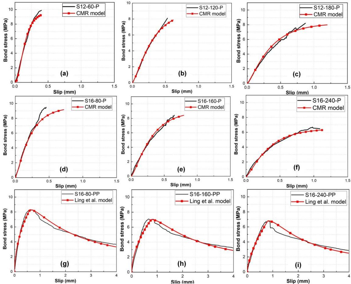
Fig. 10. Comparisons of analytical model with the average test curves
