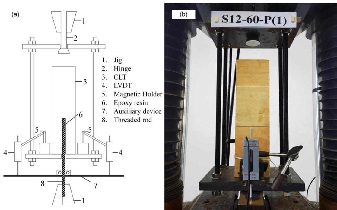
**Fig. 3.** Test set-up: (a) Schematic; and (b) photograph
