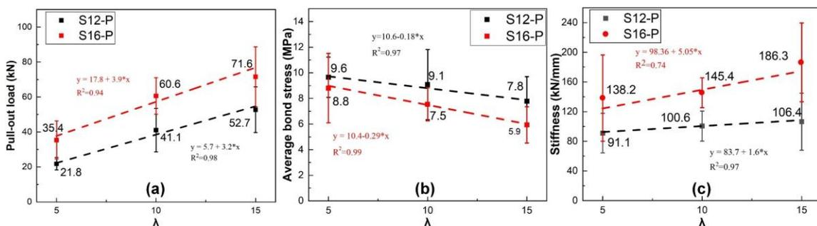
**Fig. 6.** Connection behavior at different embedment length: (a) Pull-out load; (b) Average bond stress; and (c) Stiffness
