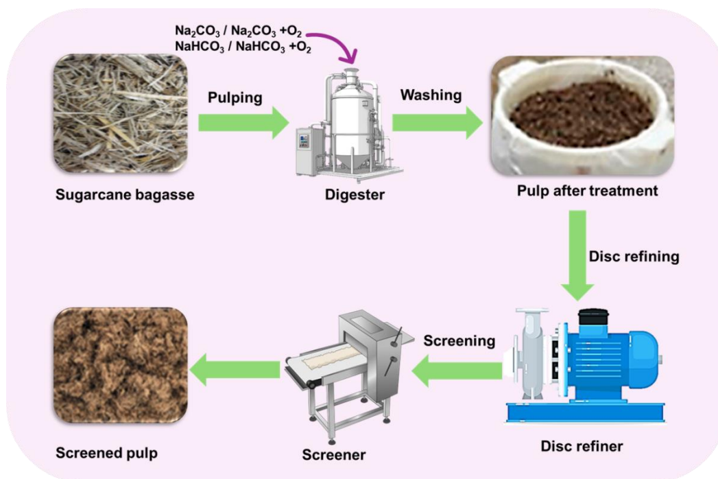
Fig. 1. Schematic representation of carbonate and bicarbonate pulping, refining and screening of the sugarcane bagasse
