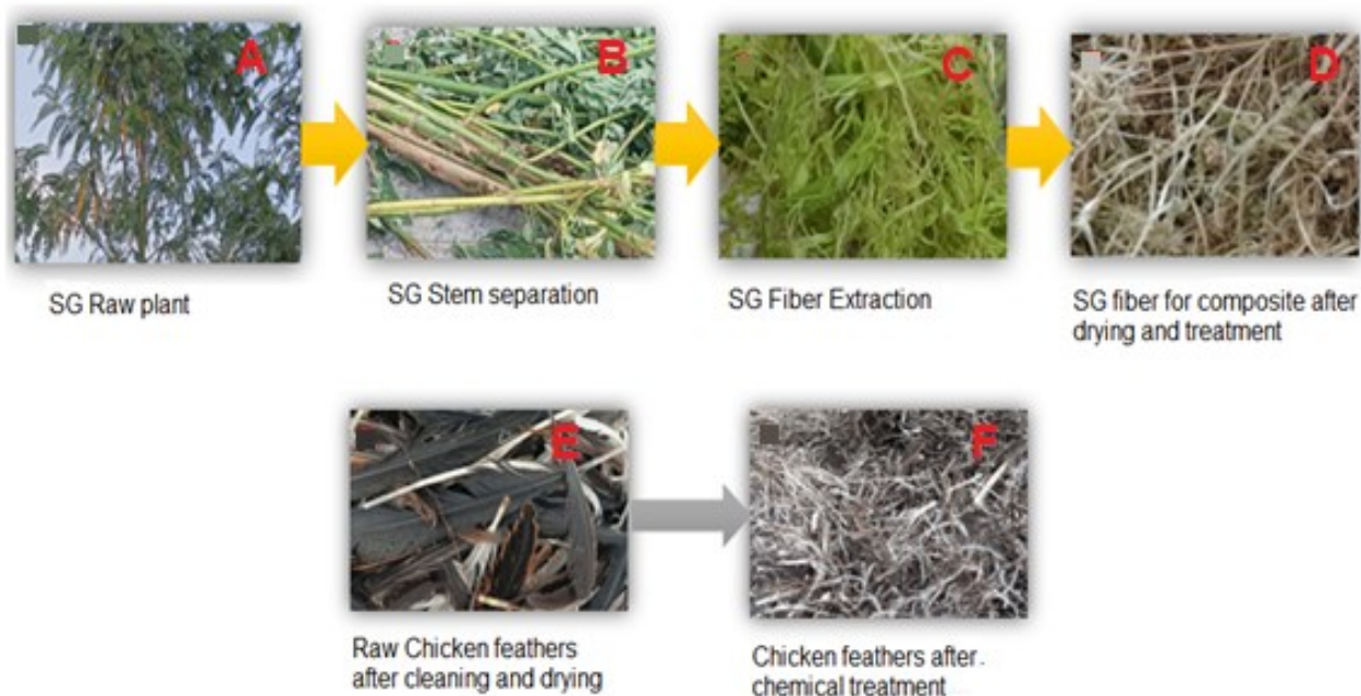
Fig. 1. Preparation of Sesbania gradiflora fiber and chicken feather fiber: A. Raw plant; B. Stem separation; C. Fiber extraction; D. Fiber for composite after drying and treatment; E. Raw chicken feathers after cleaning and drying; F. Chicken feathers after chemical treatment
