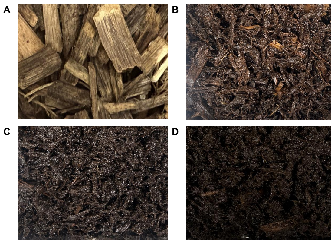
Fig. 1. Steam exploded pine wood chips. A: non-treatment; B: 225 °C, 1 min; C: 225 °C, 3 min; D: 225 °C, 5 min
