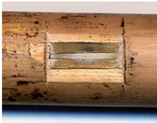
Fig. 2. A tiny free reed composed of worn coins that have been pounded into extremely thin sheets is placed inside each tube
