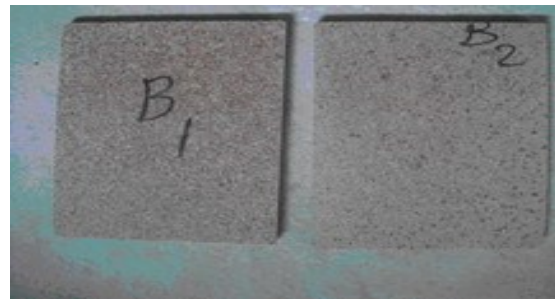
Fig. 2. Boards made from Fagus sawdust and polyethylene (B1: 40-mesh and B2: 80-mesh)
