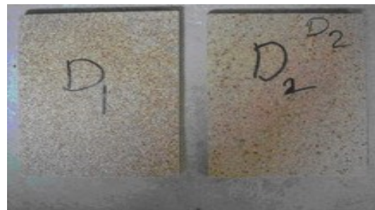
Fig. 4. Boards made from a mixture of sawdust of the above species and polyethylene (D1: 40-mesh and D2 80-mesh)
