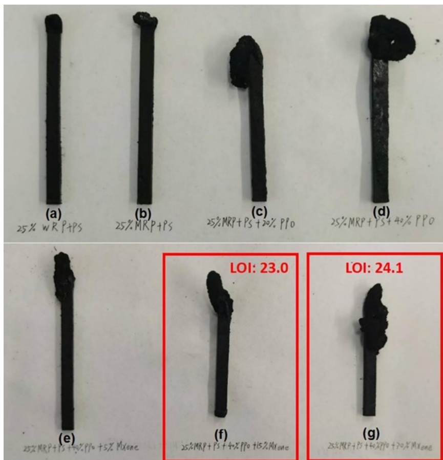
Fig. 2. Char morphology of BWTRPS, WTRPS, WTRPS/P, and WTRPS/P/M composites with LOI test (a: BWTRPS, b: WTRPS, c: WTRPS/P25, d: WTRPS/P40, e: WTRPS/P40/M5, f: WTRPS/P40/M15, and g: WTRPS/P40/M30)
