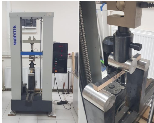
Fig. 3. Universal testing machine/three point bending test application
