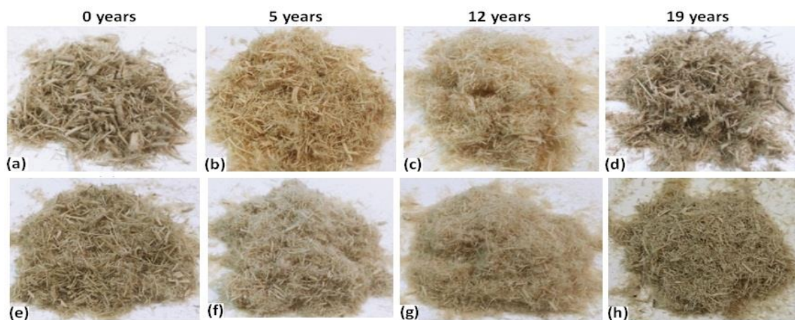
Fig. 2. Wood fiber obtained from live wood (0 years old) of Siberian fir and at different periods after its death (5 to 19 years old) after the first stage of chip preparation (a to d), and after refining (e to h)
