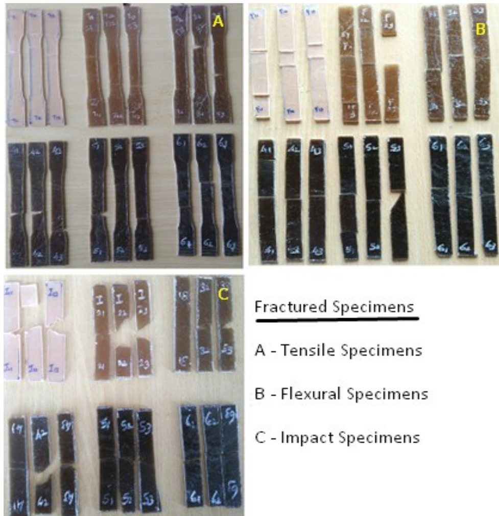
Fig. 7. Fractured Specimens: A -Tensile; B - Flexural; C - Impact
