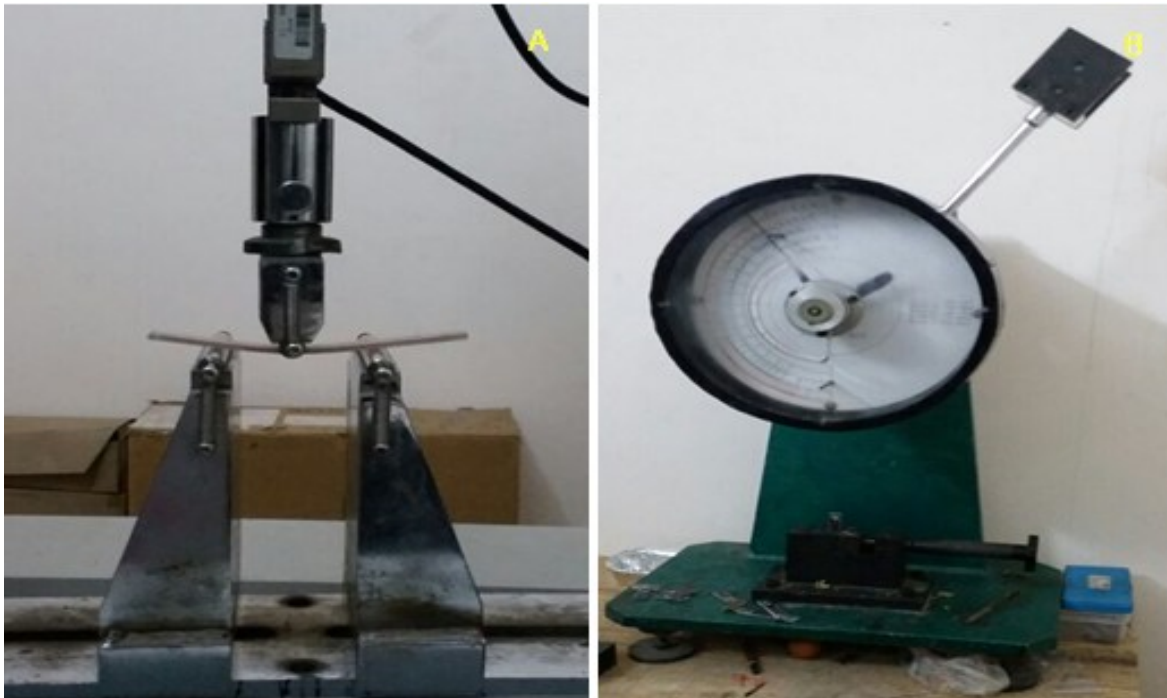
Fig. 5. A. Flexural testing samples; B. Impact testing machine
