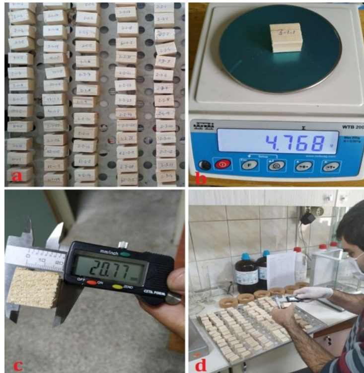
Fig. 2. Images from the work and procedures for density and sorption experiments (a,d: for shrinkage and swelling measurements, b-c: for density test)
