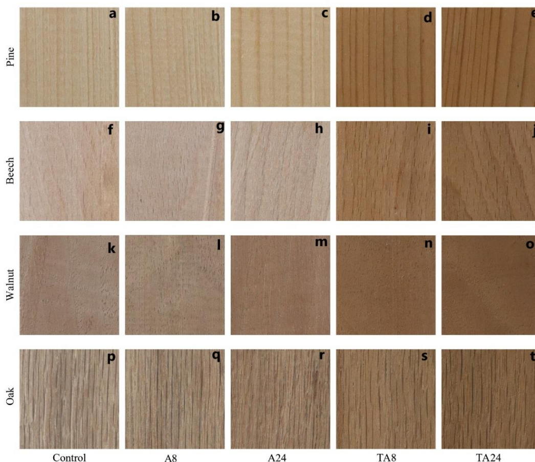
Fig. 1. Visual evaluation of control and treated wood samples with ammonia vapor and tannin
