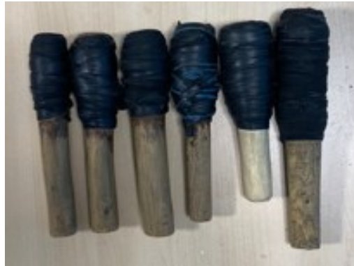
Fig. 6. The beaters made from wooden stick wrapped with rubber from motorcycle innertube
