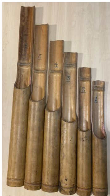
Fig. 5. The bamboo tube resonators were labelled as Tog. 1 to Tog. 6
