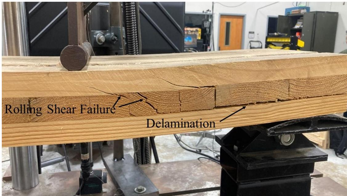
Fig. 6. Typical failure mode of treated and untreated CLT specimen
