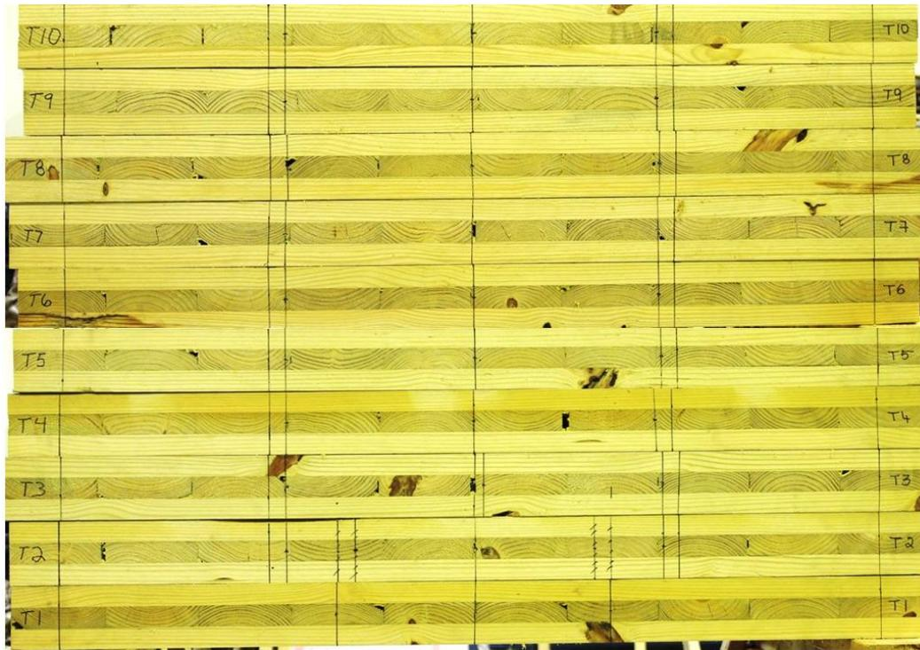
**Fig. 3.** Ten treated CLT rolling shear test specimen.
