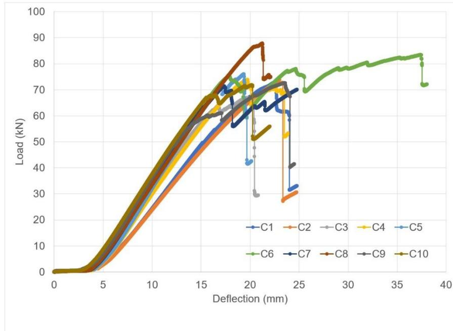
Fig. 8. Load-deflection curves of the untreated CLT specimens
