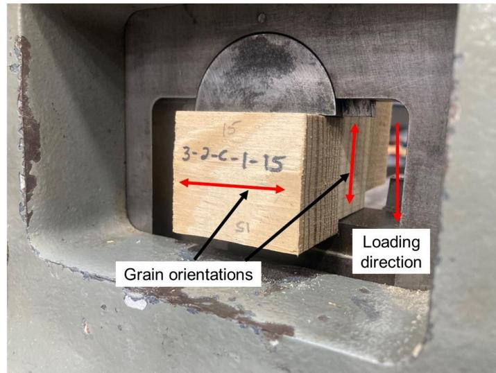
**Fig. 1.** Block shear specimen in block shear test setup.
