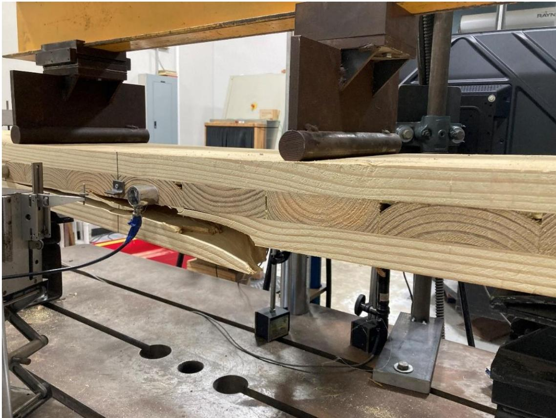
Fig. 7. Failure of bottom laminate in bending of one treated CLT specimen
