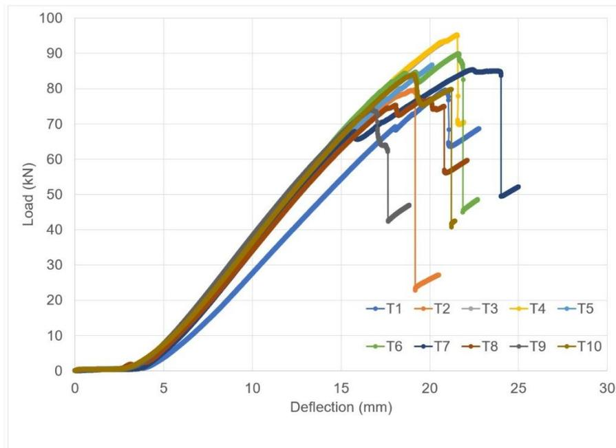
Fig. 9. Load-deflection curves of the MCA treated CLT specimens
