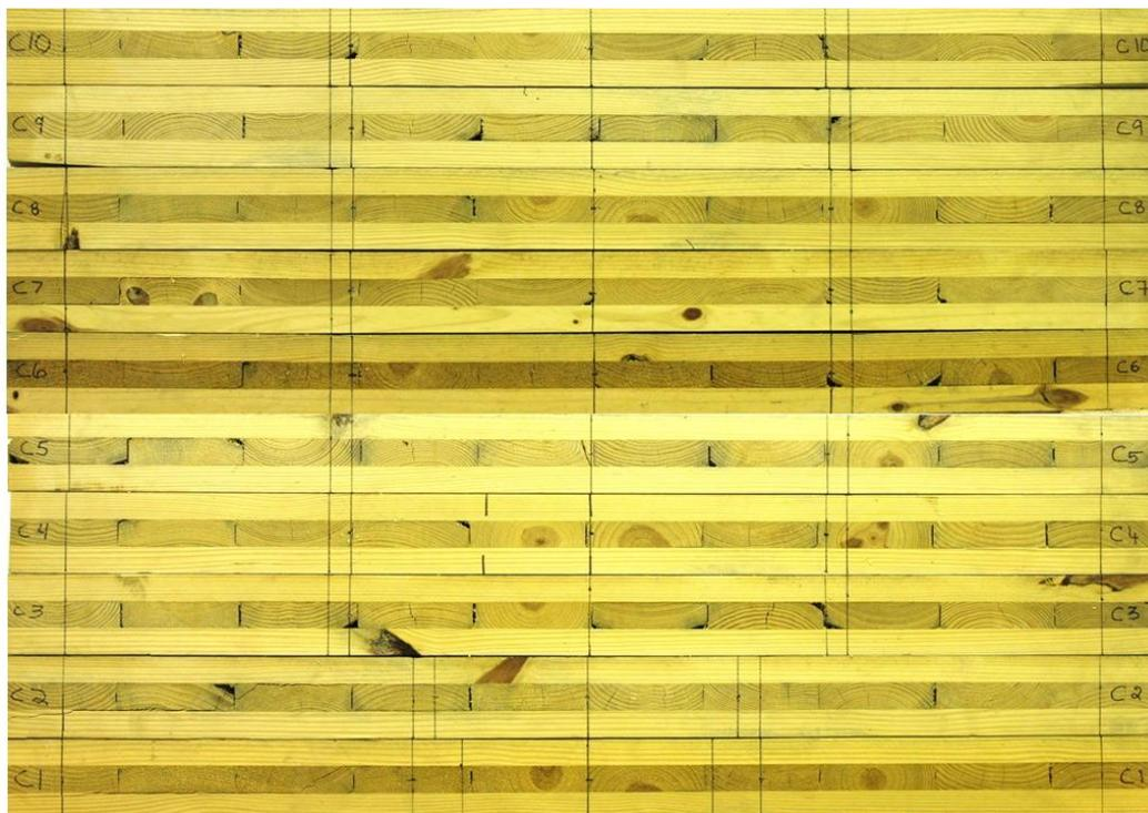
**Fig. 2.** Ten untreated CLT rolling shear test specimen
