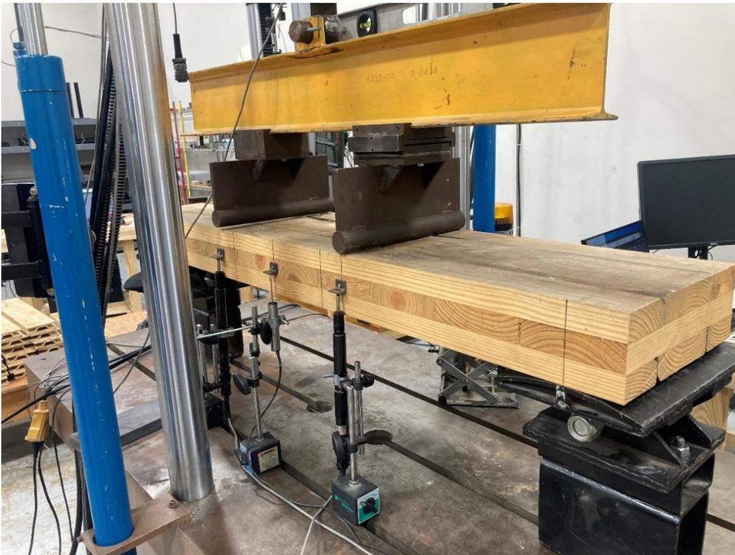
**Fig. 4.** Four-point CLT bending test setup
