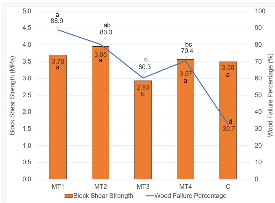
**Fig. 5.** Mean block shear strength (BSS) and wood failure percentage (WFP) (different letters above or between the numbers indicate significant differences ( $p < 0.05$ ) amount the CLT groups. Tukey Honestly Significant Difference (HSD) Test for multiple comparisons found the means values of BSS and WFP to be significantly different between some CLT groups.
