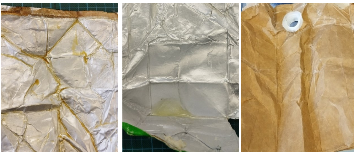
Fig. 2. Samples with residues before cleaning of inner surface (left and middle) and after cleaning (right)
