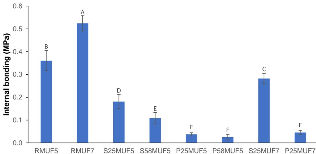
**Fig. 16.** Internal bond strength of MUF-bonded boards (letters above the error bars that are the same do not have a statistically significant difference by the Tukey's test  $\alpha = 0.05$ )
