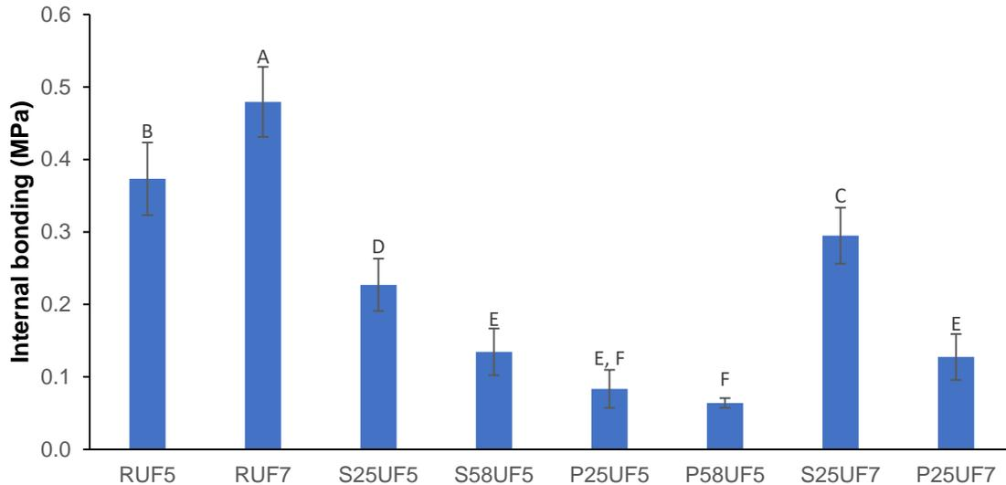
**Fig. 15.** Internal bond strength of UF-bonded boards (letters above the error bars that are the same do not have a statistically significant difference by the Tukey's test  $\alpha = 0.05$ )
