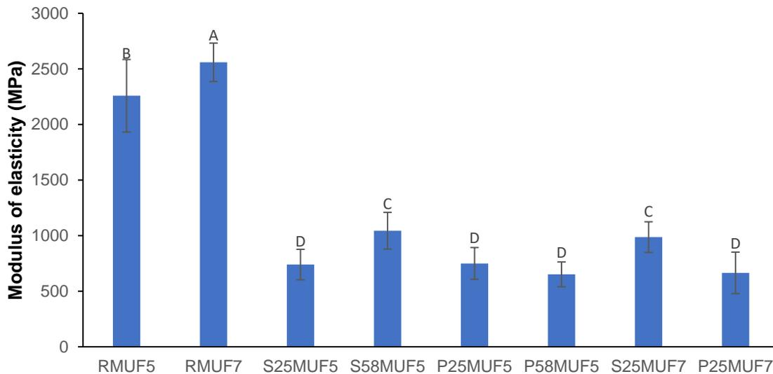
**Fig. 14.** Modulus of elasticity of MUF-bonded boards (letters above the error bars that are the same do not have a statistically significant difference by the Tukey's test  $\alpha = 0.05$ ).
