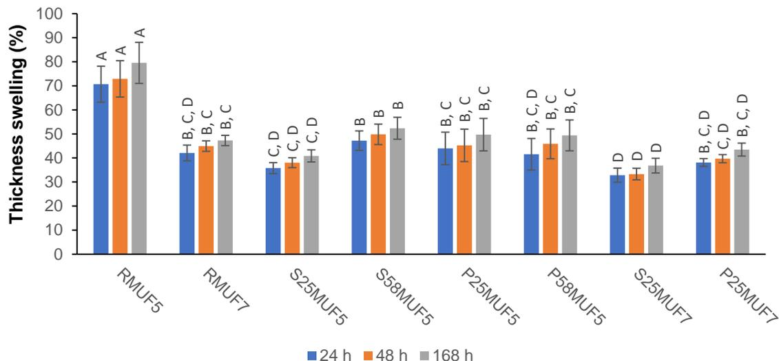
**Fig. 8.** Thickness swelling of MUF-bonded specimens after varying duration of water immersion (letters above the error bars that are the same do not have a statistically significant difference by the Tukey's test  $\alpha = 0.05$ )
