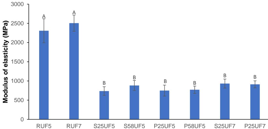
**Fig. 13.** Modulus of elasticity of UF-bonded boards (letters above the error bars that are the same do not have a statistically significant difference by the Tukey's test  $\alpha = 0.05$ ).
