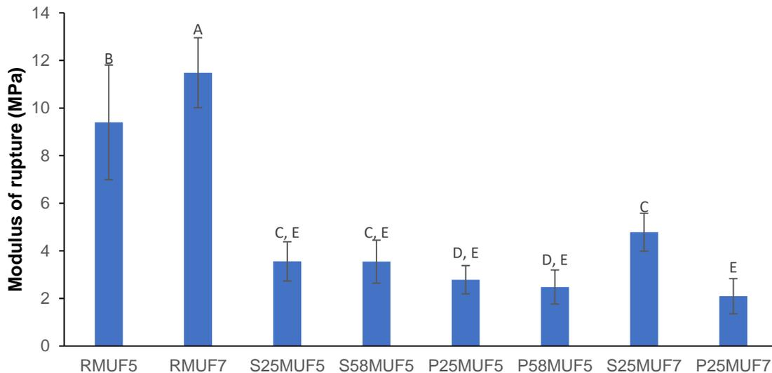
**Fig. 12.** Modulus of rupture of MUF-bonded boards (letters above the error bars that are the same do not have a statistically significant difference by the Tukey's test  $\alpha = 0.05$ )
