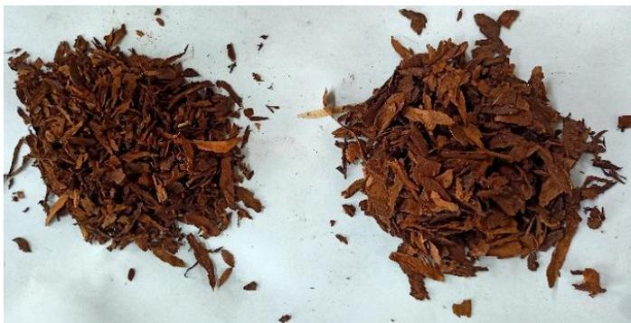
**Fig. 2.** Spruce bark particles 2 to 5 mm (left) and 5 to 8 mm (right)
