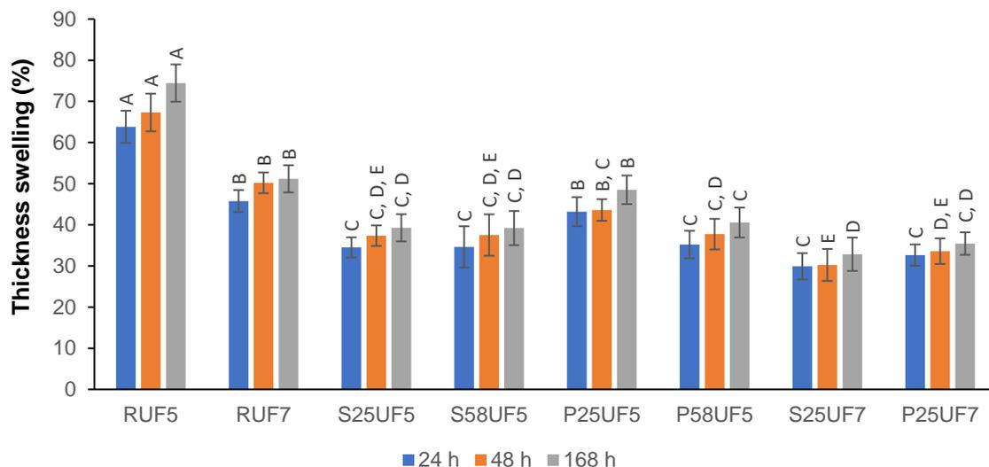
**Fig. 7.** Thickness swelling of UF-bonded specimens after varying duration of water immersion (letters above the error bars that are the same do not have a statistically significant difference by the Tukey's test  $\alpha = 0.05$ )
