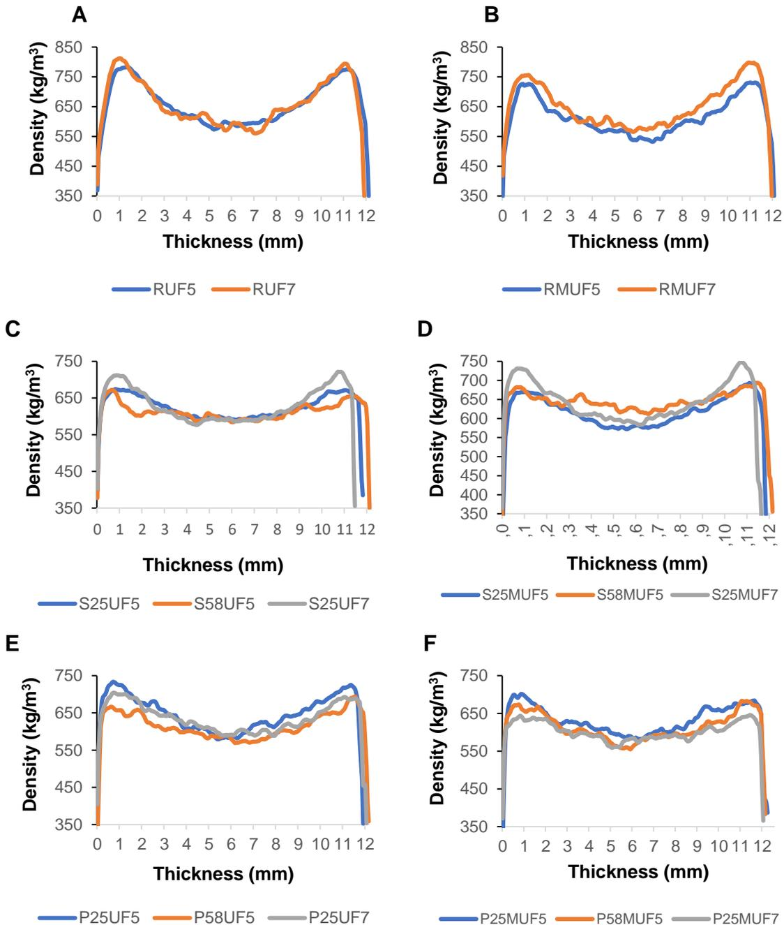
**Fig. 6.** The density profile of reference particleboards (A, B), spruce (C, D) and pine (E, F) bark boards bonded with UF (A, C, E) and MUF (B, D, F) resin
