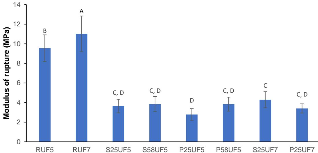
**Fig. 11.** Modulus of rupture of UF-bonded boards (letters above the error bars that are the same do not have a statistically significant difference by the Tukey's test  $\alpha = 0.05$ ).
