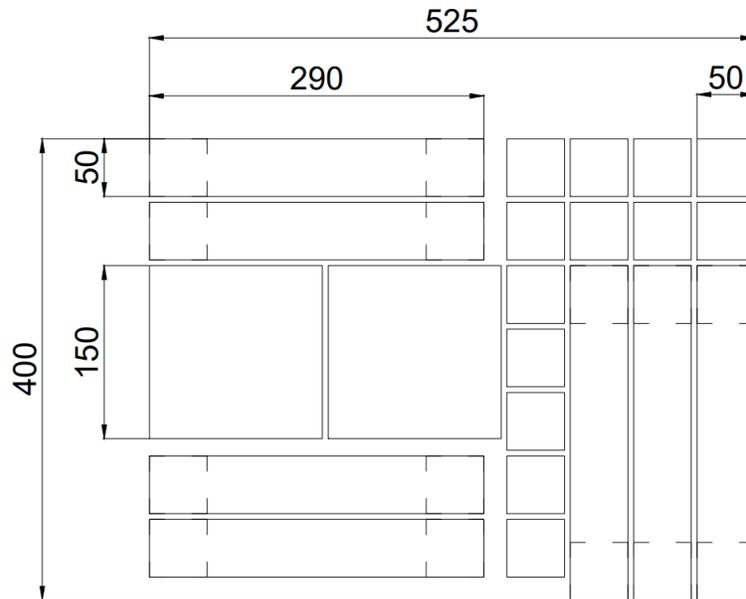
Fig. 5. Cutting plan for test specimen production
