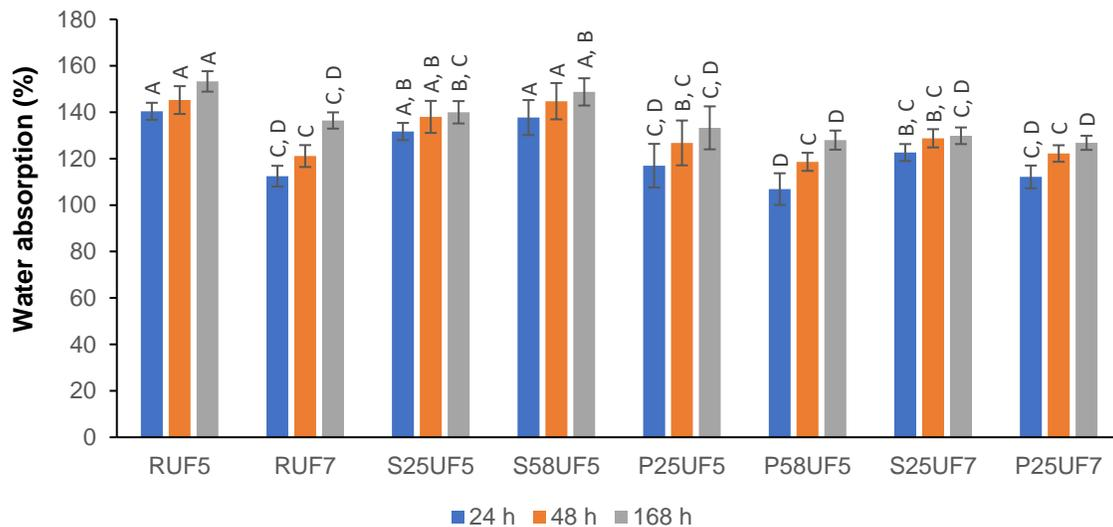
**Fig. 9.** Water absorption of UF-bonded specimens after varying duration of water immersion (letters above the error bars that are the same do not have a statistically significant difference by the Tukey's test  $\alpha = 0.05$ ).
