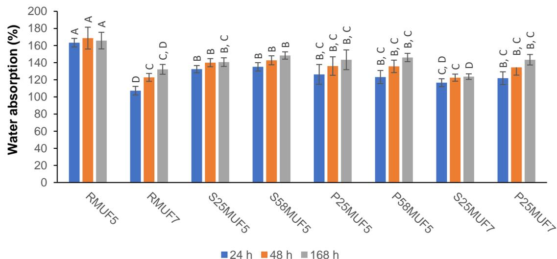
**Fig. 10.** Water absorption of MUF-bonded specimens after varying duration of water immersion (letters above the error bars that are the same do not have a statistically significant difference by the Tukey's test  $\alpha = 0.05$ ).
