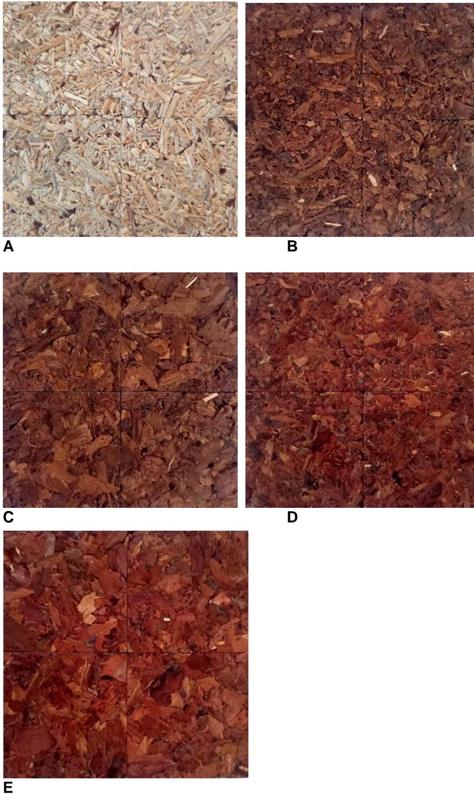
**Fig. 4.** (A) Reference particleboard made from spruce wood particles, and boards made from (B) spruce bark particles with size 2 to 5 mm, (C) spruce bark particles with size 5 to 8 mm, (D) pine bark particles with size 2 to 5 mm, and (E) pine bark particles with size 5 to 8 mm
