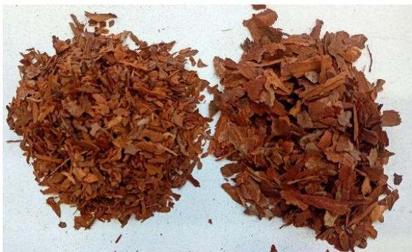
**Fig. 3.** Pine bark particles 2 to 5 mm (left) and 5 to 8 mm (right)
