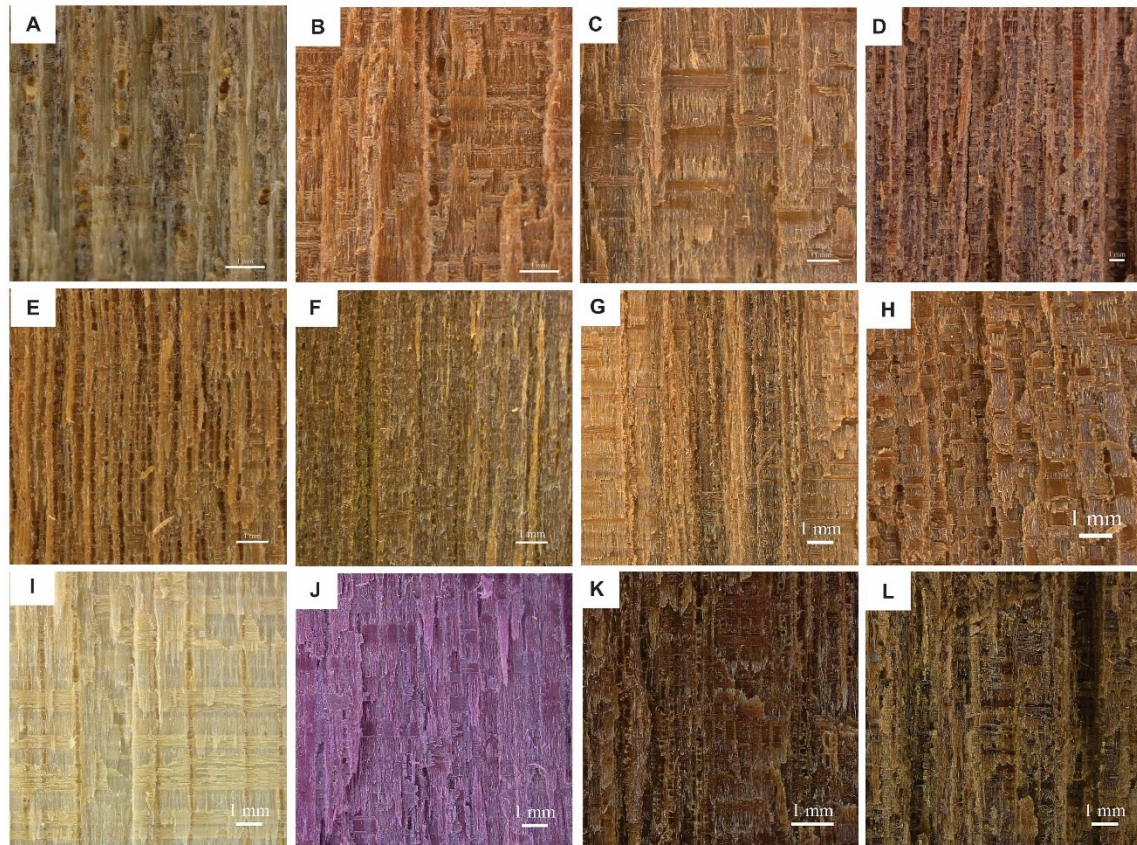
Fig. 7. Radial plane of twelve commercial wood samples from the Brazilian Amazon: (A) Amburana acreana ; (B) Cedrela sp.; (C) Hymenaea sp.; (D) Hymenolobium sp.; (E) Apuleia leiocarpa ; (F) Handroanthus sp.; (G) Astronium sp.; (H) Guarea sp.; (I) Simarouba amara ; (J) Peltogyne sp.; (K) Manilkara sp.; (L) Bowdichia sp. The black arrows on the left side of each image indicate the growth rings. A representative scale (white bar) equivalent to 1 mm is shown.
