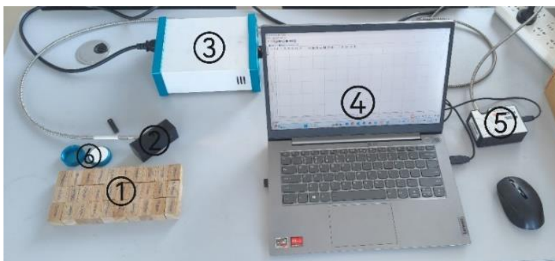
Fig. 1. Near-infrared spectral data acquisition platform for the wood samples
