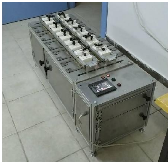
Fig. 3. The image processing-based scrub tester (IPBST)
