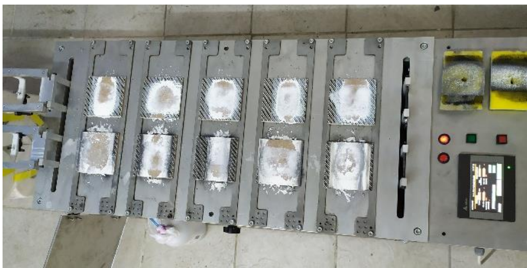
Fig. 4. Scrubbing with acetone
