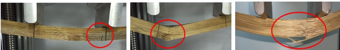
Fig. 10. Bending failure mode of laminated bamboo panels: (a) Failure caused by the glue line between bamboo and adhesive; (b) fracture due to the splintering tension; (c) failure due to compression buckling and tension; (d) rolling shear failure; (e) failure due to brittle fracture
