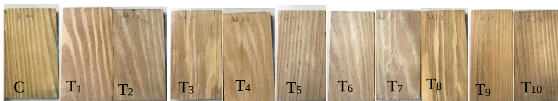
Fig. 1. Appearance quality of ACQ-D with different treatments without outdoor exposure (C) and after one year outdoor exposure (T1-T10)
