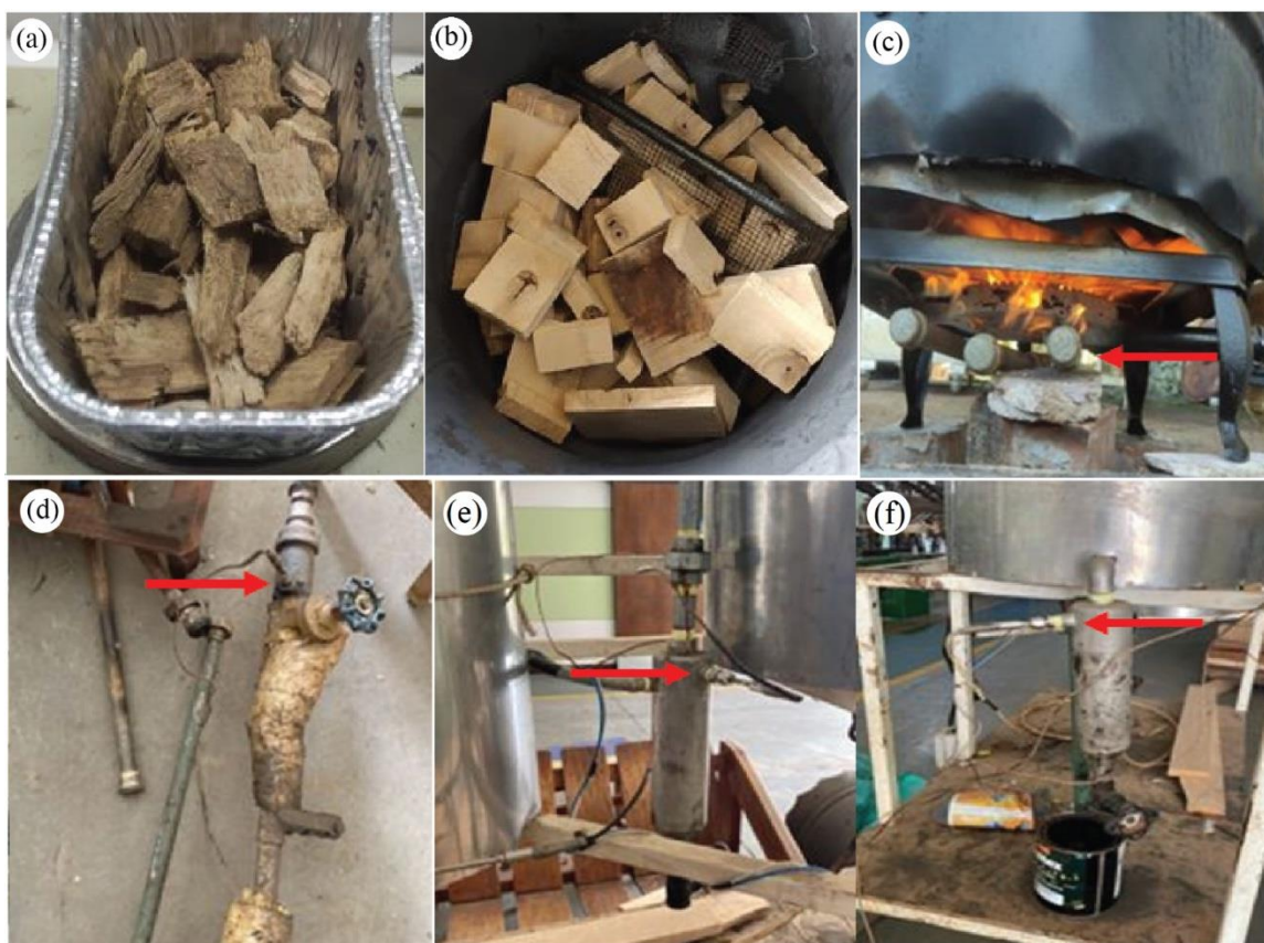
Fig. 1. Wood residues of G. arborea used in the pyrolysis process: (a) wood chips and (b) solid board-ends; Different parts in the reactor: Non-condensable gases outlet (c) and temperature meter probes at three stages of the wood residues pyrolysis process: pyrolyzer gas outlet (d), after the first cooler (e) and after the second cooler (f)
