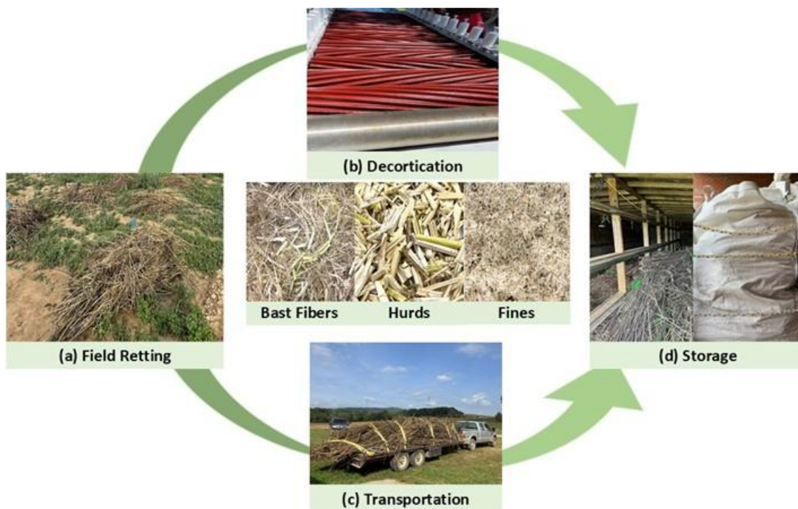
Fig. 6. A representation of industrial hemp post-harvest handling and processing operations (a) field retting, (b) decortication, (c) transportation, and (d) storage
