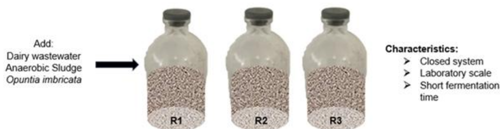
Fig. 2. Schematic design of batch reactors (triplicate)
