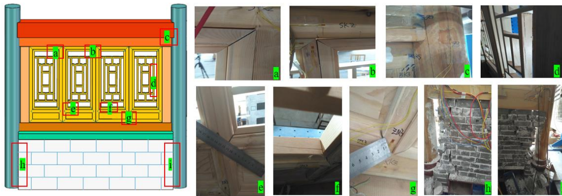
Fig. 9. Damages of Kanchuang (displacements 150 mm): (a) tenon of Shangmo pulled out of the mortise; (b) compression of wood; (c) compression of Fang; (d) Lingtiao split; (e) Xiamo pulled out of mortise; (f) Crack of Zaibian; (g) tenon of Xiamo pulled out of the mortise; (h) left side of the wall collapsed; (i) right side of the wall collapsed
