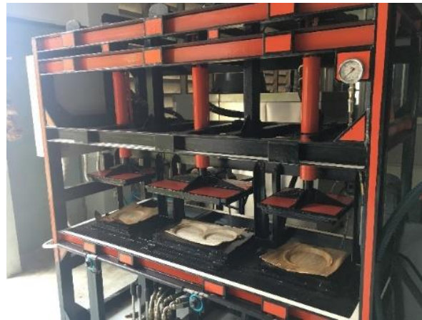
Fig. 5. The bag of arecanut leaves used the hot plate of the hydraulic packing machine
