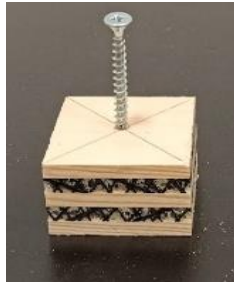
Fig. 4. Withdrawal resistance of single screw example
