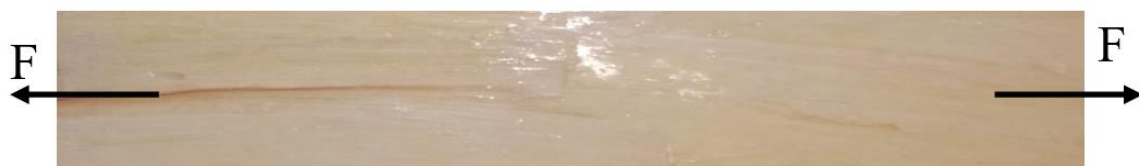
Fig. 4. An example of the tensile test conducted along the fibers of the sample
