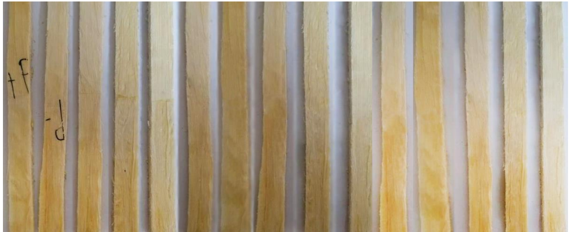
Fig. 3. An illustrative case that involves the 15 specimens, which were cut from the A30 group, prepared specifically for the tensile test
