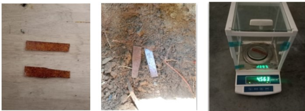
Fig. 11. Biodegradability test for cork-epoxy composite
