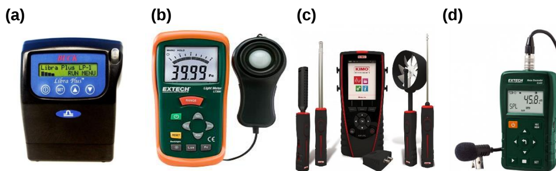
Fig. 1. Occupational hygiene measurement devices, (a) personal dust exposure measurement device, (b) lighting measurement device, (c) thermal comfort measurement device, (d) personal noise exposure measurement device
