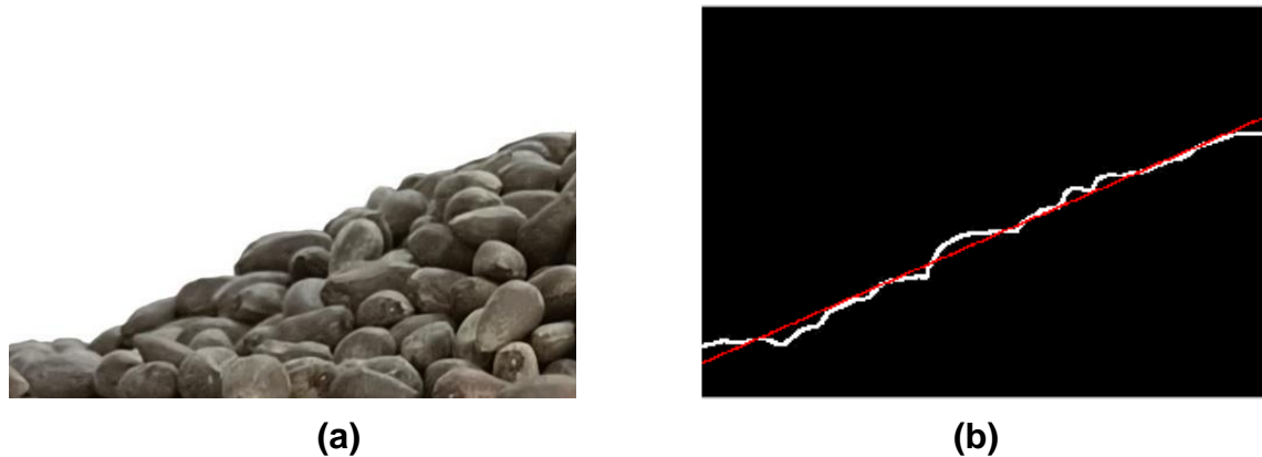
Fig. 7. Image processing of repose angle measurement of cottonseed. (a) Original image; (b) Contour extraction and line fitting
