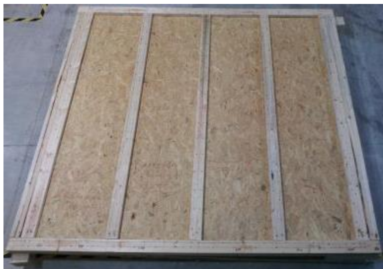
Fig. 14. The midply shear wall connected by wood nails
