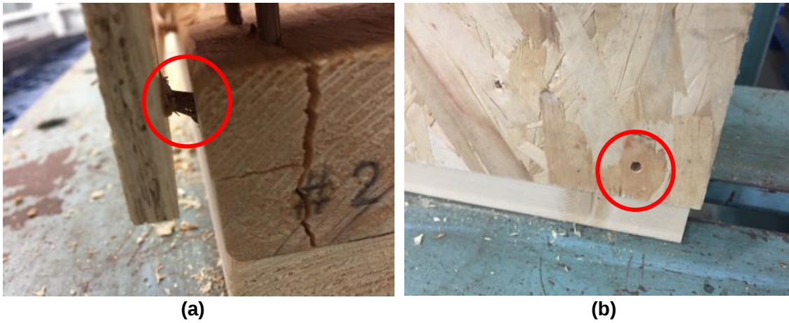
Fig. 6. The bent (a) and indentation (b) of the wood nails
