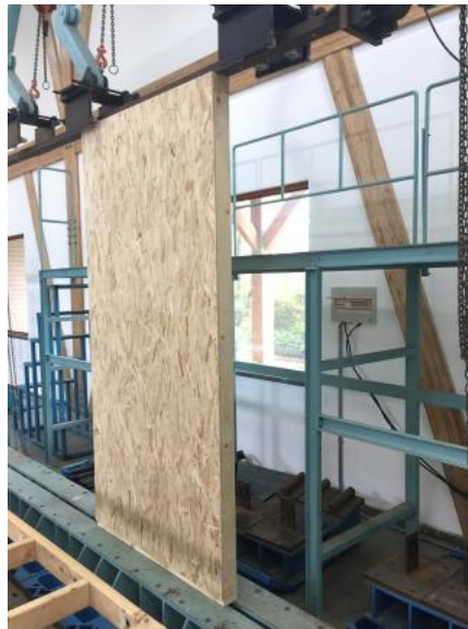
Fig. 5. The shear wall fixed to the testing system
