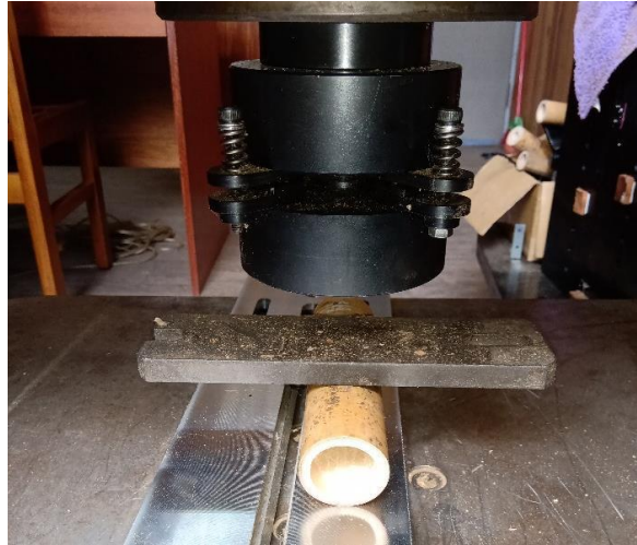
Fig. 4. Lateral partial compression test
