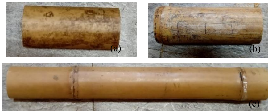
Fig. 3. None-node compression specimen (a), one-node compression specimen (b), two-node compression specimen (c)
