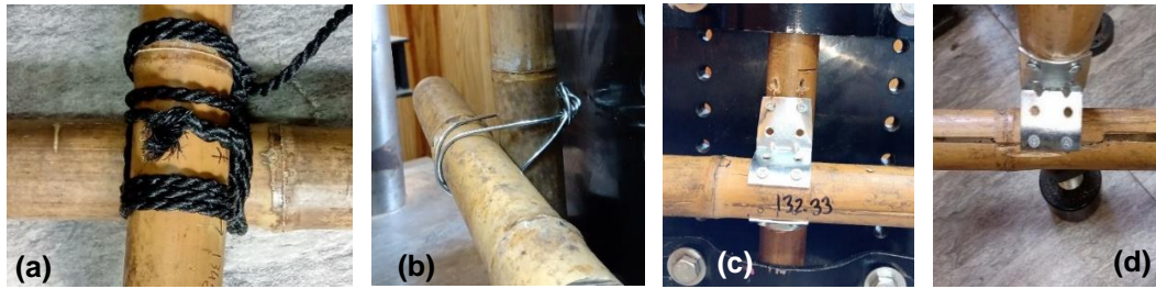
Fig. 13. Failure mode of slip test in a lashing joint with node (a), iron wire joint (b) and steel angle bracket joint (c and d)
