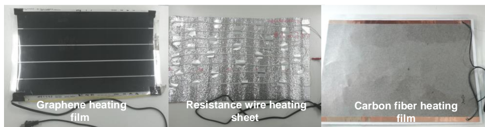
Fig. 1. Materials of heating layer
